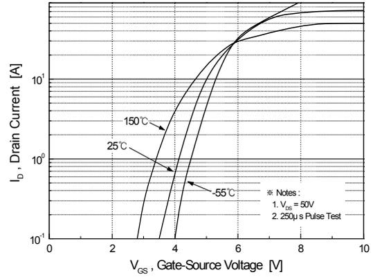
Figure 2. Transfer Characteristics
