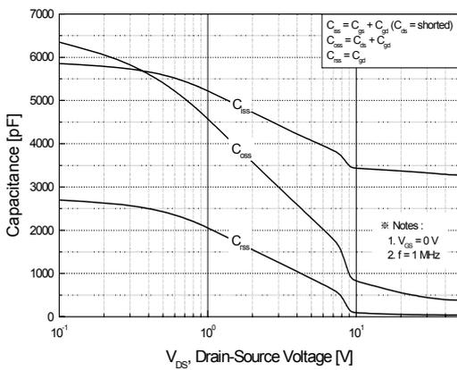
Figure 5. Capacitance Characteristics
